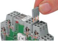
Easy commoning using adjacent jumpers
