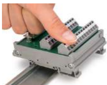
Snapping a module onto DIN-rail.
