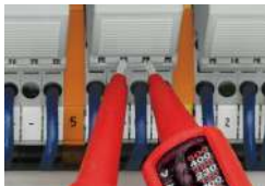
Function testing via touch-proof test slots
