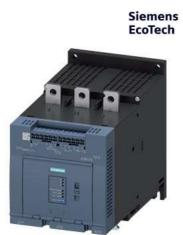
SIRIUS soft starter 200-480 V 470 A, 24 V AC/DC Spring-loaded terminals Thermistor input
