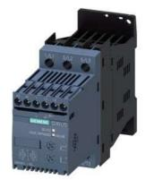
SIRIUS soft starter S00 6.5 A, 3 kW/400 V, 40 °C 200-480 V AC, 24 V AC/DC Screw terminals
