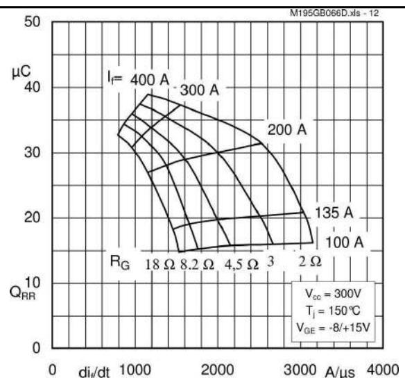
Fig. 12 Typ. CAL diode recovered charge
