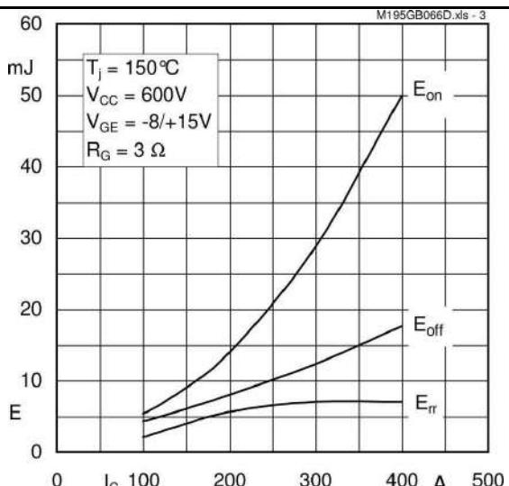
Fig. 3 Typ. turn-on /-off energy =  $f (I_C)$
