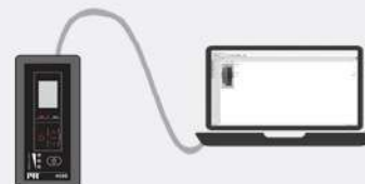
Connection of ConfigMate 4590 to a PC in Docking Mode
