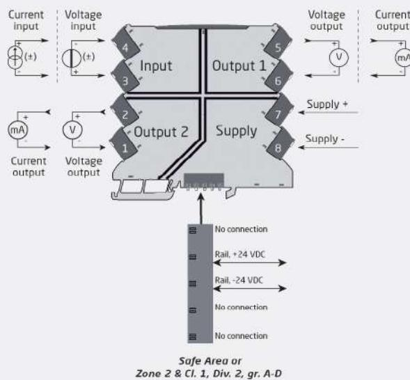
(\* ) Bipolar Input to bipolar output wiring set-up:
