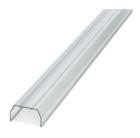
Cover profile, for covering terminal strips, snaps onto cover profile carrier AP 3-TU, AP 3-TNS 35, can be marked with insert strip AP-ES. Cover profile carriers should be placed at the ends and at intervals of approx. 40 cm. Length: 1 m
