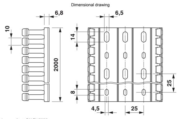
Base perforation according to DIN EN 50085
