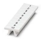
Zack marker strip, Strip, white, labeled, Printed vertically: consecutive numbers 1 ... 10, 11 ... 20, etc. up to 91 ... 100, mounting type: snapped, for terminal block width: 3.5 mm, lettering field size: 3.5 x 10.5 mm, Number of individual labels: 10
