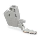
Pick-off terminal, nom. voltage: 1000 V, nominal current: 32 A, number of connections: 1, connection method: Screw connection, cross section:  $0.14 \text{ mm}^2 - 6 \text{ mm}^2$ , mounting type: on base element, color: gray
