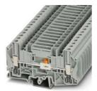
Disconnect terminal block, with spring support, nom. voltage: 1000 V, nominal current: 41 A, connection method: Screw connection, 1 level, Rated cross section: 6 mm², cross section: 0.2 mm² - 10 mm², mounting type: NS 35/7,5, NS 35/15, NS 32, color: gray
