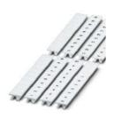
Marker for terminal blocks, Strip, white, labeled, can be labeled with: CMS-P1-PLOTTER, horizontal: L1, L2, L3, N, PE, L1, L2, L3, N, PE, mounting type: snapped, for terminal block width:  $8.2\,$  mm, lettering field size:  $10.5\,$ x  $8.15\,$ mm, Number of individual labels:  $10\,$
