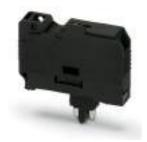
Fuse plug, Prior to replacing the cartridge fuse, disconnect the fuse connector from the basic terminal block., nominal current: 10 A, connection method: Plug-in connection, fuse type: G /  $6.3 \times 32$ , mounting type: Plug-in mounting, color: black
