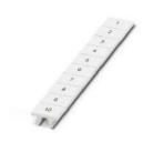
Zack marker strip, Strip, white, labeled, can be labeled with: CMS-P1-PLOTTER, Printed vertically: consecutive numbers 1 ... 10, 11 ... 20, etc. up to 91 ... 100, mounting type: snapped, for terminal block width: 8.2 mm, lettering field size: 10.  $5 \times 8.15$  mm, Number of individual labels: 10
