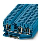
Feed-through terminal block, nom. voltage: 1000 V, nominal current: 57 A, number of connections: 3, connection method: Spring-cage connection, 1 level, Rated cross section: 10 mm<sup>2</sup>, cross section: 0.2 mm<sup>2</sup> - 16 mm<sup>2</sup>, mounting type: NS 35/7,5, NS 35/15, color: blue
