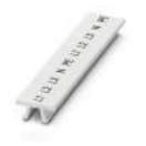
Zack marker strip, Strip, white, labeled, horizontal: L1, L2, L3, N, PE, L1, L2, L3, N, PE, mounting type: snapped, for terminal block width: 5.2 mm, lettering field size: 5.15 x 10.5 mm, Number of individual labels: 10
