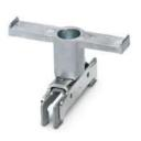
Support bracket, Bracket for busbars, set every 20 cm, depth: 33.7 mm, width: 56 mm, height: 50 mm, number of positions: 2, color: silver, mounting type: DIN rail mounting
