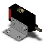
Medium Photoelectric Sensor With Built-in Amplifier, Diffuse-reflective, Horizontal, Sensing distance: 200 mm, NPN, Timer/Self diagnosis function, Turbo function, Pre-wired model, 2 m
