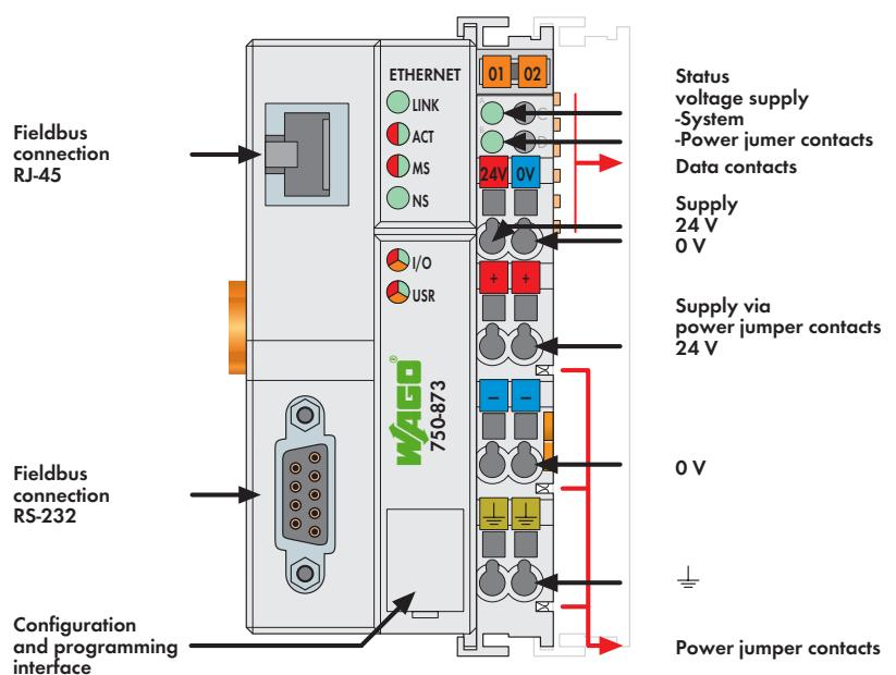
This PLC connects ETHERNET to the WAGO-I/O-SYSTEM. The controller automatically configures, creating a local process image which may include analog, digital or specialty modules. Analog and specialty module data is sent via words and/or bytes; digital data is sent bit by bit. The IEC 61131-3 programmable controller is capable of 10/100 Mbit/s data rates, providing 512 KB program memory, 256 KB data memory and 24 KB retain memory. It has a battery-backed RTC and 32-bit multitasking CPU.
