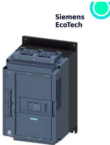
SIRIUS soft starter 200-480 V 47 A, 110-250 V AC Screw terminals Analog output
