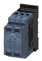
SIRIUS soft starter S3 106 A, 55 kW/400 V, 40  $^{\circ}\text{C}$  200-480 V AC, 24 V AC/DC spring-type terminals Thermistor motor protection
