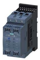
SIRIUS soft starter S3 106 A, 55 kW/400 V, 40 °C 200-480 V AC, 24 V AC/DC Screw terminals Thermistor motor protection
