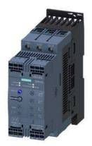
SIRIUS soft starter S2 72 A, 37 kW/400 V, 40  $^{\circ}\text{C}$  200-480 V AC, 24 V AC/DC spring-type terminals Thermistor motor protection
