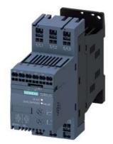
SIRIUS soft starter S00 12.5 A, 5.5 kW/400 V, 40 °C 200-480 V AC, 110-230 V AC/DC spring-type terminals
