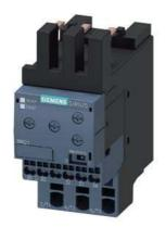
Monitoring relay, can be mounted to Contactor 3RT2, Size S0 basic, analog adjustment Apparent current monitoring 4...40 A, 50...60 Hz, 2-phase Supply 24-240 V AC/DC 1 change-over contact Monitoring for Current overshoot and undershoot Phase failure, Cable break with or without fault buffer ON delay 0-60 s Noise pulse suppression 0-30 s Switching hysteresis 6% spring-type connection system
