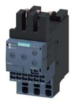
Monitoring relay, can be mounted to Contactor 3RT2, Size S0 basic, analog adjustment Apparent current monitoring 4...40 A, 50...60 Hz, 2-phase Supply 24 V AC/DC 1 change-over contact Monitoring for Current overshoot and undershoot Phase failure, Cable break with or without fault buffer ON delay 0-60 s Noise pulse suppression 0-30 s Switching hysteresis 6% spring-type connection system
