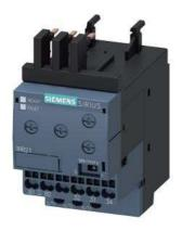
Monitoring relay, can be mounted to Contactor 3RT2, Size S00 basic, analog adjustment Apparent current monitoring 1.6-16 A, 20-400 Hz, 2-phase Supply 24-240 V AC/DC 1 change-over contact Monitoring for Current overshoot and undershoot Phase failure, Cable break with or without fault buffer ON delay 0-60 s Noise pulse suppression 0-30 s Switching hysteresis 6% spring-type connection system
