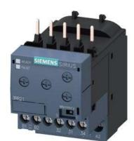
Monitoring relay, can be mounted to Contactor 3RT2, Size S00 basic, analog adjustment Apparent current monitoring 1.6-16 A, 20-400 Hz, 2-phase Supply 24-240 V AC/DC 1 change-over contact Monitoring for Current overshoot and undershoot Phase failure, Cable break with or without fault buffer ON delay 0-60 s Noise pulse suppression 0-30 s Switching hysteresis 6% Screw connection system
