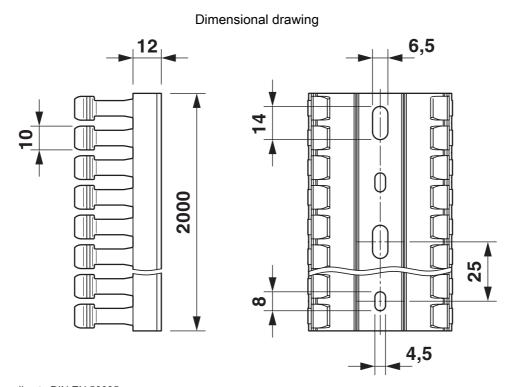
Base perforation according to DIN EN 50085
