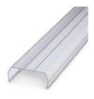
Cover profile for covering terminal strips, snaps onto cover profile carrier APT-ME or end clamp APH-ME. A cover profile carrier is to be positioned at the ends and at intervals of around 40 cm. Length as per customer requirement.
