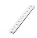
Marker for terminal blocks, Strip, white, labeled, can be labeled with: CMS-P1-PLOTTER, horizontal: L1, L2, L3, N, PE, L1, L2, L3, N, PE, mounting type: snapped, for terminal block width: 10.2 mm, lettering field size:  $10,15 \times 10,5 \text{ mm}$ , Number of individual labels: 10
