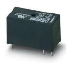
Plug-in miniature solid-state relay, power solid-state relay, 1 N/O contact, input: 5 V DC, output: 24 - 253 V AC/2 A
