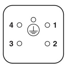
Connector pin assignment connection side: Left pin; right socket
