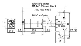
Note 3: SM2S-05B: 83.3 max., SM2S-05C: 83.3 max., SM2S-05D: 88.3 max.,SM2S-05DF: 88.3 max. Note 4: SM2S-05B: 86.8 max., SM2S-05DF: 86.8 max., SM2S-05D: 91.8 max.,SY4S-05DF: 91.8 max.
